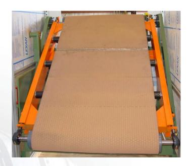
The Three Position Sorting Conveyor features fully pneumatic positioning and electric tire handling for superb repeatability. Completely setup and configured through the intuitive TIGRE program. The sorter comes complete with all necessary hardware and includes side safety guarding.
